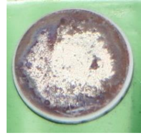
Figure 75. Performed first attempts at characterizing mechanical properties of lithium films post electrochemical cycling.
