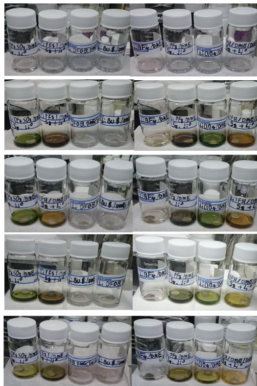
Figure 105. DME-based electrolytes with elemental sulfur contacted with lithium metal at different times.
