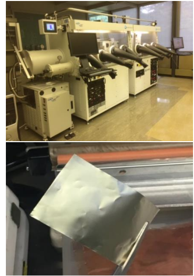
Figure 55. PVD system integrated with glovebox for making lithium thin-film electrode and protective coatings.
