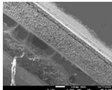
Figure 1. Cross section of a dry electrode.
