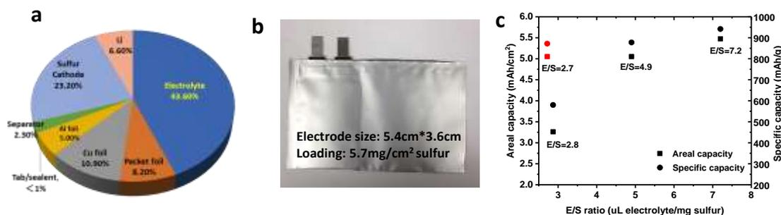
**Figure 91.** (a) Component weight distribution of Li-S battery with energy density of 300 Wh/kg. (b) Photo image of single-layer pouch cell used in present study (electrode working area 19.4 cm<sup>2</sup>, and sulfur mass loading 5.7 mg/cm<sup>2</sup>). (c) Dependence of first discharge areal capacity and specific capacity on electrolyte/sulfur ratio (black symbol: pouch cell using pristine separator; red symbol: pouch cell using modified separator).
