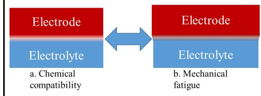
This project will be focusing on the interfacial design to improve the chemical stability and mechanical stability of electrode/electrolyte interface for efficient mass transport of lithium ions for all solid state batteries.
