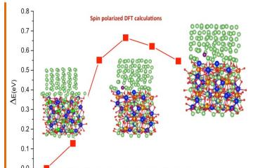
Figure: Energy barrier obtained from density functional theory lithium atom migration from LLZO to lithium metal. The magnitude of the barrier obtained is 0.65 eV.
