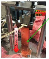
Sample placed between Cu bars Temperature drop measured
