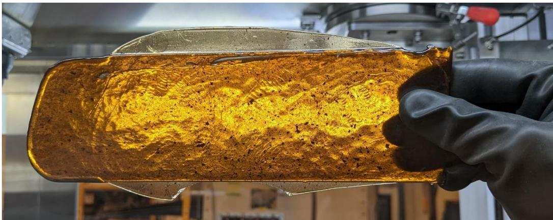
Figure 13. ISU-6 preform made using new high-quality small-scale synthesis route.
