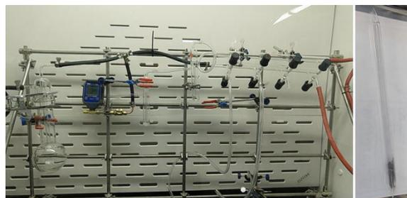
Figure 3. Digital photo of vacuum sealing set up for the synthesis of solid-state electrolytes.
