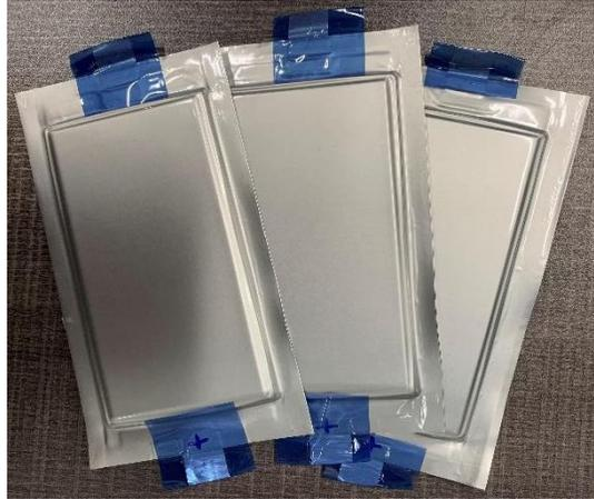
Figure 22. All-solid-state 2-Ah Li-NMC pouch cells.
