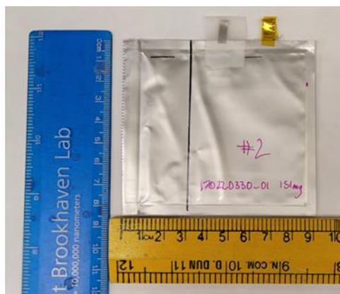
Figure 167. Single-layer pouch cell using baseline electrode.
