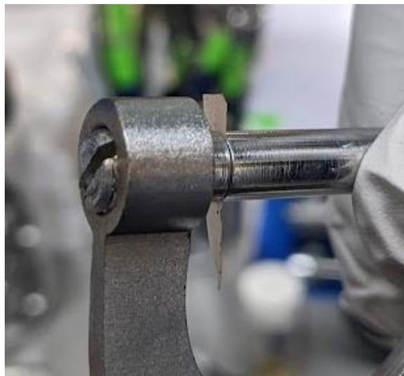
Figure 14. Image of 60- $\mu\text{m}$  thin film in a micrometer.
