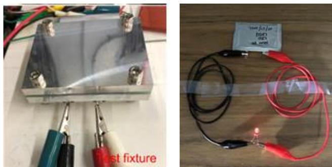
**Figure 39.** (left) All-solid-state pouch cell (full cell, 2 × 3 inch), and (right) cell under test in a pressure fixture.
