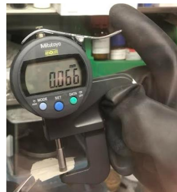
Figure 7. Photograph of a thin, freestanding sulfide solid-state electrolyte separator measured by thickness gauge.
