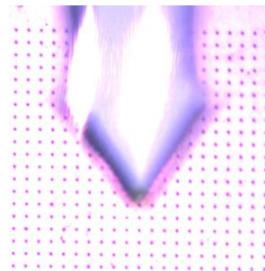
Task 2.2 – Figure 1. Optical image of custom silicon nitride window to be capped with graphene and holes filled with liquid electrolyte.
